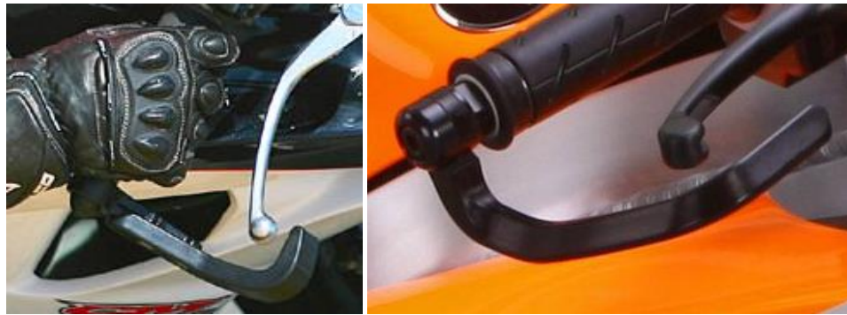
Picture 15 - Examples of front brake lever protections
